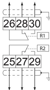
In case of inductive loads on the relay outputs, protective wiring must be provided (e.g. RC or diode arc suppression)
