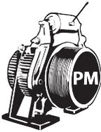
When using PM motors, the encoder position/pole must also be learned. This step is unique to PM applications and does not need to be done with IM machines. Knowing the motor pole position relative to the encoder allows the KEB drive to apply the proper stator magnetic field commutation angle for maximum torque.
