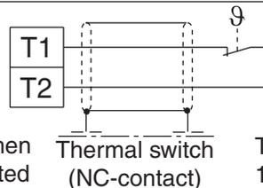
Thermal switch (NC-contact)
