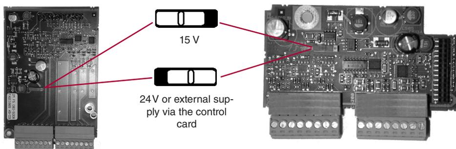
The maximum load capacity is dependent on the selected voltage supply.
