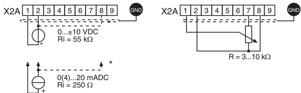
Connect unused analog inputs to common to eliminate noise signals!
