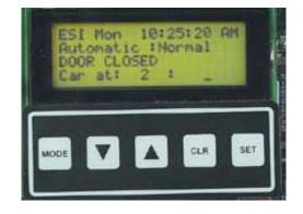
**MODE**: Used to change LCD Display Mode.
