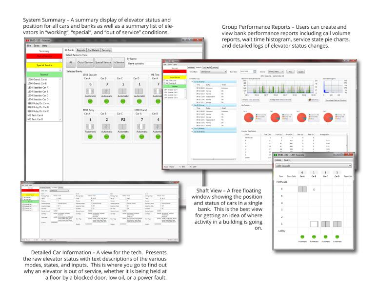
EMIS 100 can be configured to display a pop-up message or audible alert when an elevator goes out of service.
