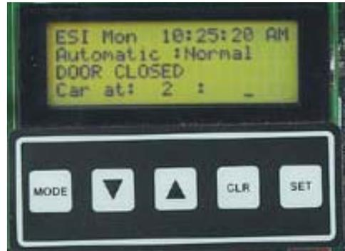
**MODE** : Used to change LCD Display Mode.
